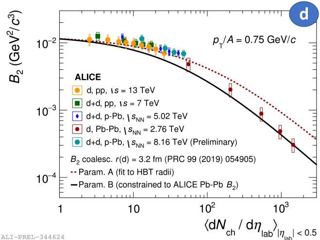
Strong dependence of  $B_2$  on collision system size
