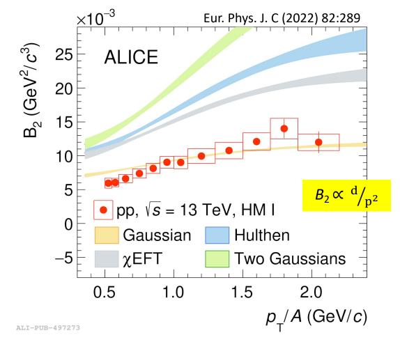
$$B_2(p_T)pprox rac{3}{2m}\int d^3q D(q)e^{-R_{p_T}^2q^2} \ D(q)=\int d^3r|\phi_d(r)|^2e^{-iq\cdot r} \ egin{align*} & ext{Blum, Takimoto} \ & ext{PRC 99 (2019) 044913} \ & ext{deuteron wave function} \ & ext{(size $d=3.2$ fm)} \ \end{pmatrix}$$
