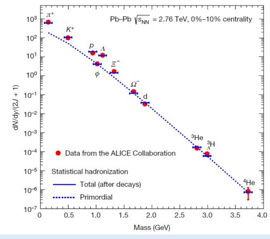
→ In Pb–Pb collisions, particle yields of light-flavour hadrons are described over 9 orders of magnitude with a **common** chemical freeze-out temperature of  $T_{\text{chem}} \approx 153 \text{ MeV}$ .
