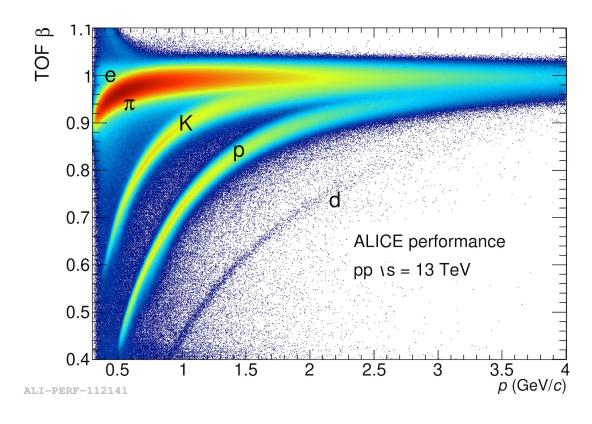
Higher p region (above 1 GeV/c)  $\rightarrow$  PID via velocity  $\beta$  measurements in TOF
