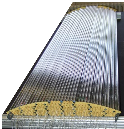
Outer sector module consisting of 7 layers
