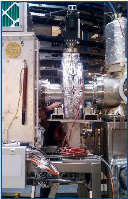
New sensitive Schottky cavity Resonance frequency 410 MHz
