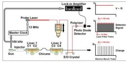
prototype monitor for electron bunch form and arrival time in cw linacs
