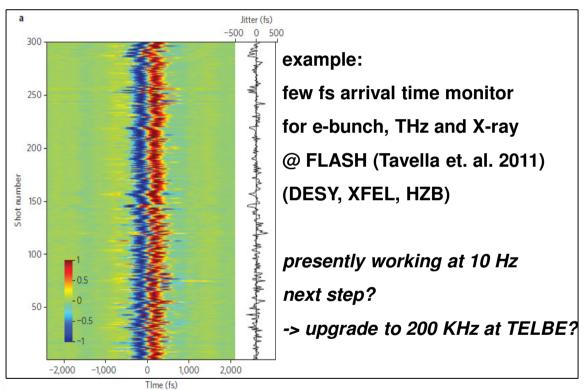
far goal is fast feedback and single bunch /pulse diagnostic at high rep rates (KHz – MHz)
