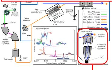
BECOLA is the first (still the only) **collinear laser spectroscopy** setup at an in-flight facility.
