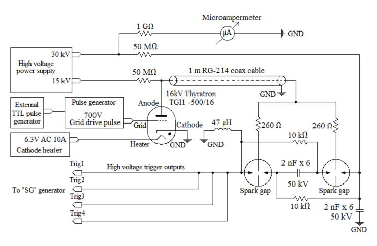
The trigger generator is a two-stage Marx generator with an output capacitance of 6 nF. Each stage consists of six low inductance ceramic high-voltage capacitors (2 nF, 50 kV) connected in parallel and two gas spark switches with central electrodes at half the charging voltage.
