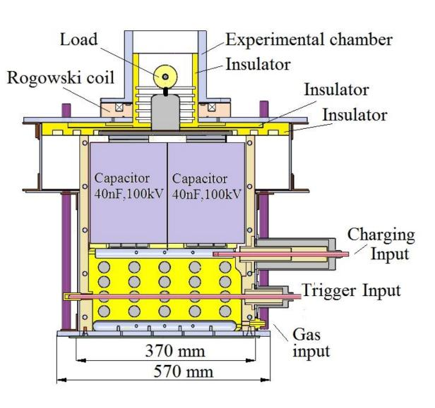
The SG generator consists of four bricks. Each brick consists of two low-inductance HV capacitors (40 nF, 100 kV, 15 nH) connected in parallel and a multigap, multichannel ball gas spark switch with capacitively coupled triggering.
