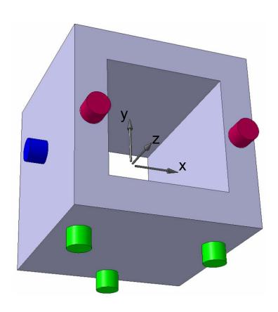
For a 3-D object there are 6 degrees of freedom in the Cartesian coordinate system: displacements dx, dy, dz and rotations rx, ry, rz.
