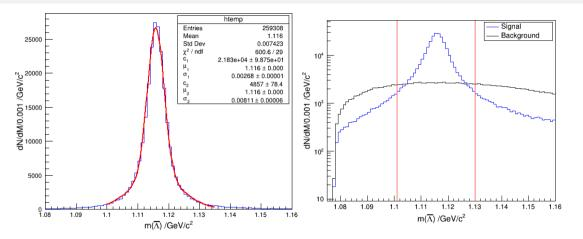
Mass Resolution:  $\sigma_{m_{fit}}(\bar{p}\pi^+) = 2.680 \cdot 10^{-3} \text{ GeV/c}^2$ , Mass Window:  $|m_{\text{fit}}(\bar{p}\pi^+) - m_{\text{PDG}}(\bar{\Lambda})| < 5 \cdot \sigma_{m_{fit}}(\bar{p}\pi^+)$
