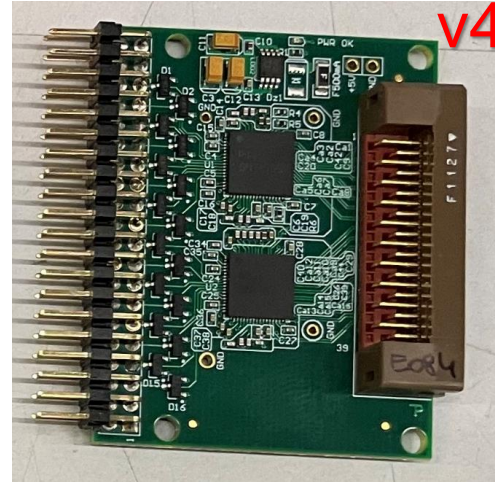
PASTTREC board (v3) with bonded ASICs (left) and new board (v4) with packed ASICs (middle). Exchange of faulty boards at STS1 by new boards (right).
