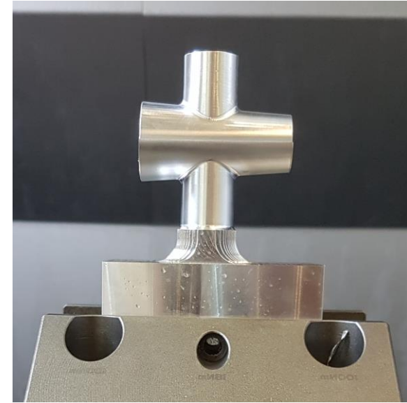
Picture 2: IP-cross – conical D_{\text{inner}} 20 mm to 28 mm
