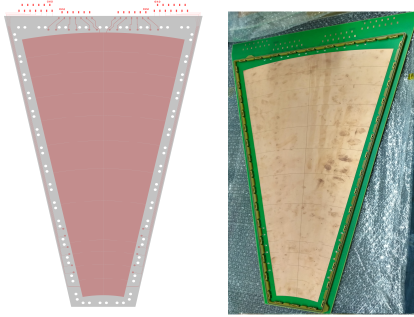
Figure 5.1: Left: Gerber layout of real-size drift PCB with HV connections. Right: Picture of fabricated drift PCB with outer frame and spring contact soldered
