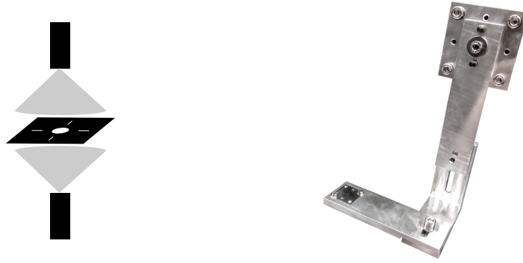
Figure 5.7: Sketch of the camera calibration setup (left). Both the top and bottom camera detect the calibration pattern simultaneously. The mounting device developed for inserting the calibration pattern in between the cameras is shown on the right.
