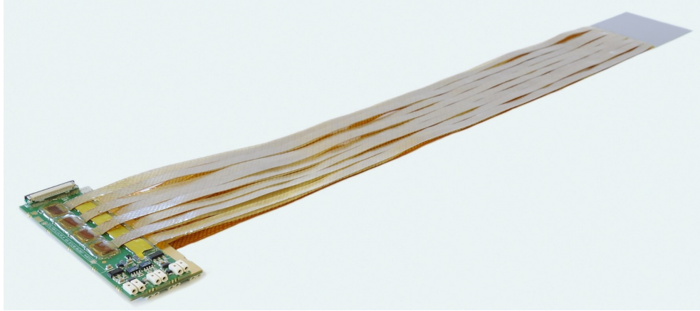
Figure 3.6: STS detector module comprising 50 cm aluminium microcables and a 6.2 cm × 6.2 cm sensor. Image courtesy of GSI.
