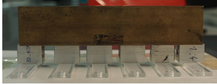
Figure 4.21: Sample preparation for underfill radiation hardness tests.
