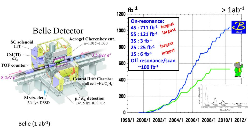
General purpose detector, built to test Standard Model mechanism for *CP* violation in *B* decays to charmonium  $(B^0 \to c\bar{c}K_S^0)$ .
