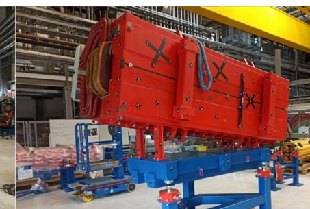
Vertical deflecting dip10 at GSI
