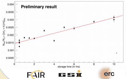
The adjacent figure shows the preliminary results from the first direct measurement of the half-life of bare <sup>205</sup>Tl ions. Longer measured half-life corresponds to a slower reduction of <sup>205</sup>Pb due to the electron capture from the 2.3 keV excited state. This is crucial for the understanding of the fate of <sup>205</sup>Pb in the early solar system.
