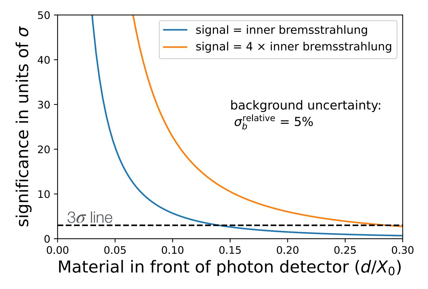
Inner bremsstrahlung (pp, 13 TeV, based on charged particles from PYTHIA 8):
