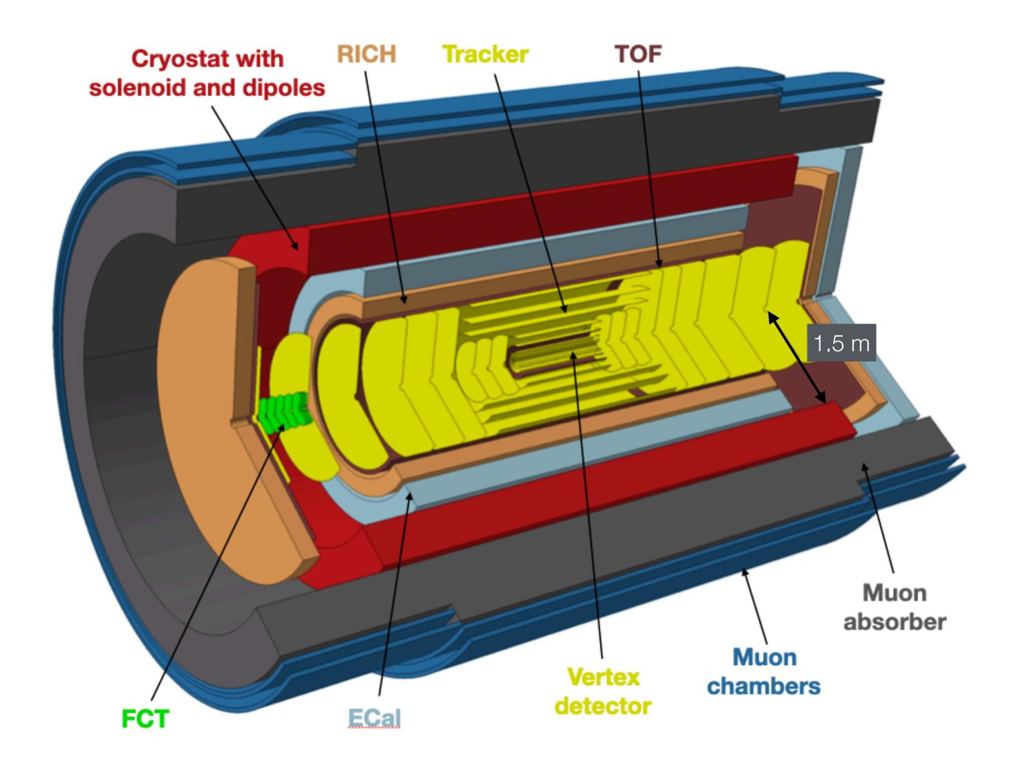
Tracking of electrons/positrons from photon conversions directly in front FCT in dipole field
