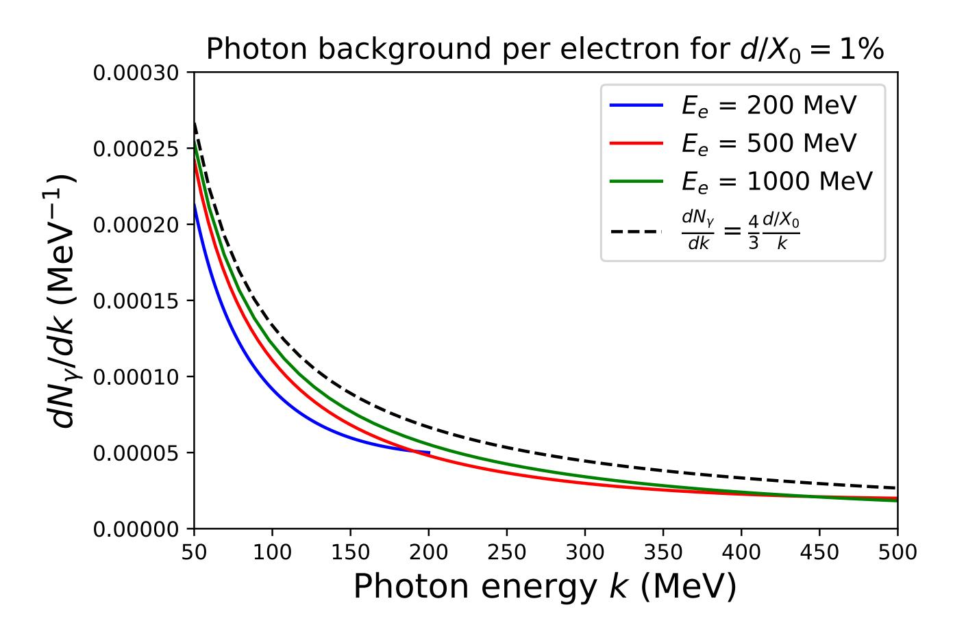
Energy spectrum of bremsstrahlung photons (from particle data book):
