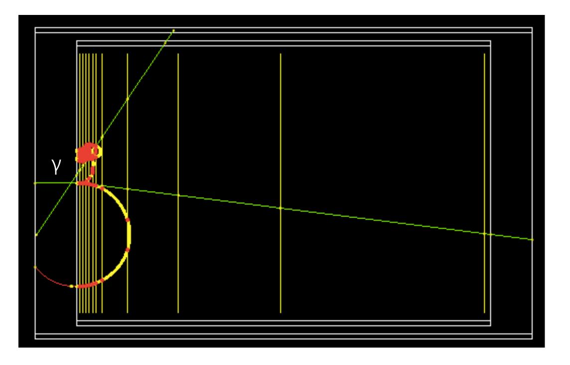
Can measure photons through conversions down to  $E_{\gamma} = 50-100 \text{ MeV}$
