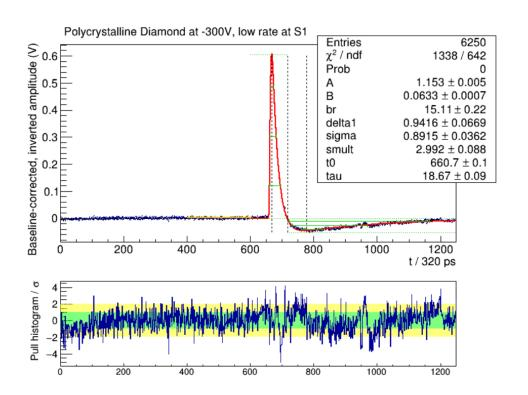
Fit quite successful (98.2%) on the first bunch of waveform before high rate irradiation
