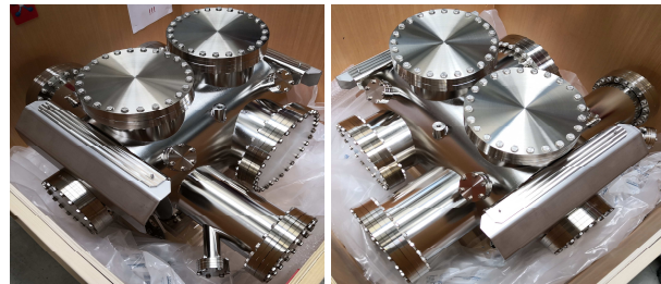
Figure 1: SIS100 laser vacuum chamber ( Kurt J. Lesker )
