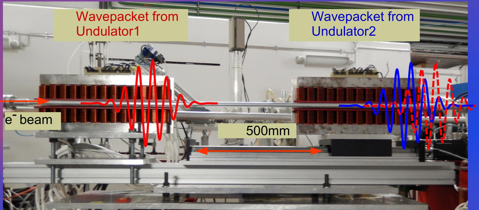
To Measure the oszillation period the second undulator ist moved by a motorized stage
