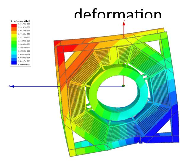
Deformation plot for the Cryostat-Iron assembly Maximum iron deformation is 3.6mm at the upper corner The maximum Cryostat deformation is ~2.5mm
