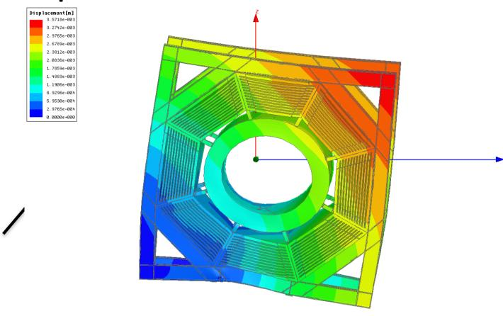
Deformation plot for the Cryostat-Iron assembly Maximum iron deformation is 3.5mm at the upper corner
