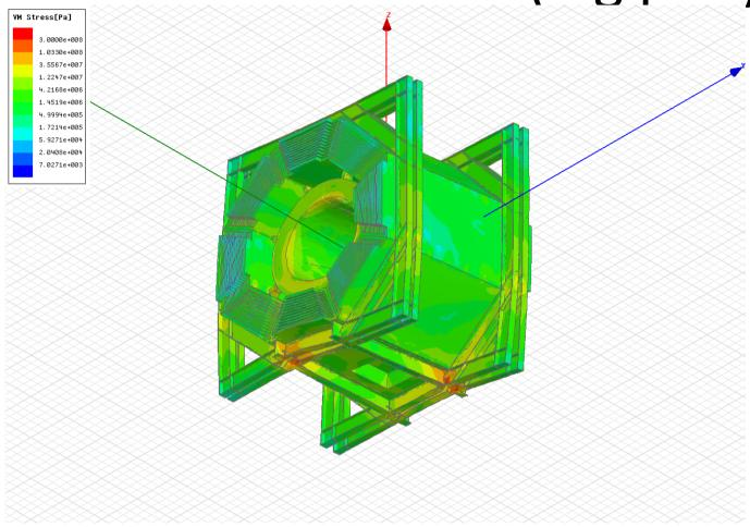
High stresses > 300 MPa are found close to the "foots"; In the rest of the iron the stresses are < 100 MPa
