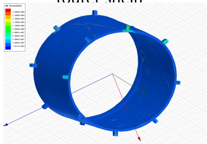
Stresses are everywere in the low scale values, on the Cryostat suspensions values are still around 100 Mpa.
