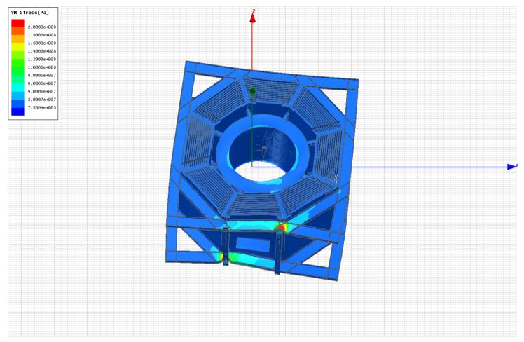
Linear plot of the von Mises stresses on the coil iron assembly in the range 7.5e3-2e8 Pa. Showing the stress concentration in the beam frame (already unrealistic) stresses on the cryostat and cryostat iron connections are in the quite safe operation limit.
