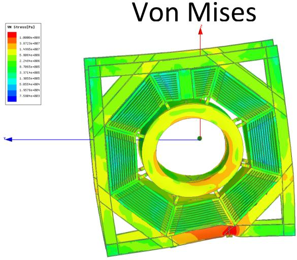
Log Plot of von Mises Stresses ranging from 7.5e3 to 1e8 [Pa] The stresses are >100M Pa in the red region at the Lower support Beam intersection. Maximum stresses on the Cryostat and Cryostat connections are below 20 [Mpa] the maximum Value on the connection is a numeric artifact produced by the coarse mesh.
