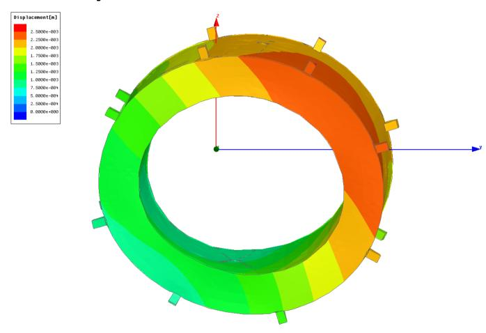
The maximum Cryostat deformation is ~2.5mm
