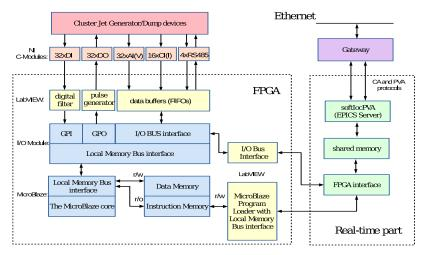
A suggested scheme of incorporating the MicroBlaze processor into NI-9039 cRIO FPGA.
