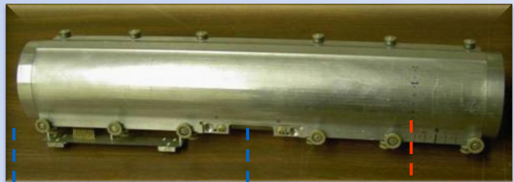
Trolley with matrix of 17 NMR Probes
