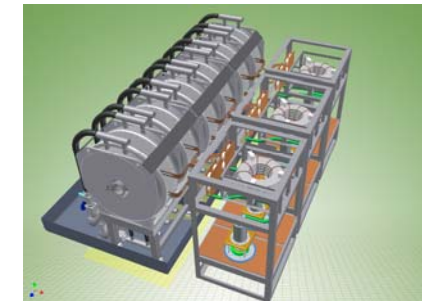
h=2 acceleration cavity for faster ramping
