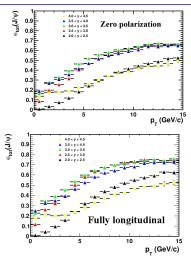
• Deviation from zero polarization gives the major systematic uncertainty ( $\sim 20\%$ ). Polarization measurement is fundamental to reduce the uncertainty.
