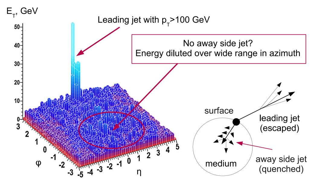
Sample di-jet event reconstructed by ATLAS in central Pb+Pb collision
