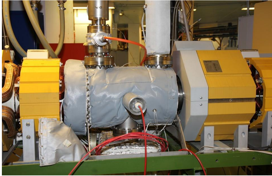
Fig. 6.7. Photograph of vacuum tank with electrostatic septum, with bakeout jacket installed.
