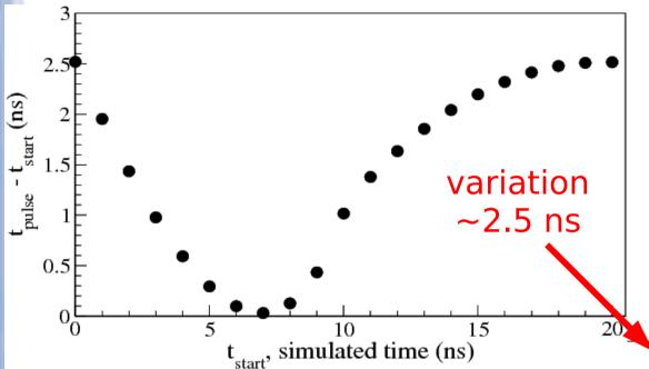
Optimization of CFT Ratio allows to reduce the variation and symmetrize the shape of the variation dependence on the phase
