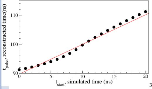
Ratio of CFT is optimized for the narrowest  $\Delta t$  distribution for pulses with same phase
