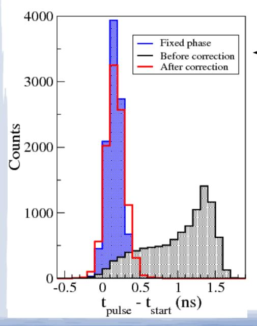
Distribution of  $\mathbf{t_{pulse}}$ - $\mathbf{t_{start}}$  obtained for random  $\mathbf{t_{start}}$  values
