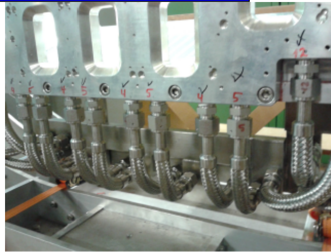
Connectors to cooling lines within mounting plate
