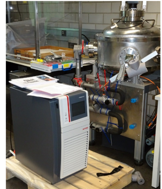
UFO test stand with the new chiller
