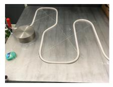
Special ATLAS (inner tracker)-approved, fast UV-ray curing glue (Dymax 6-621) to bond to aluminum front plate
