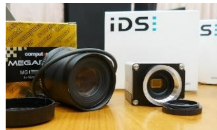
Scintillating screens: manufactured plates, received objectives & CCDs
