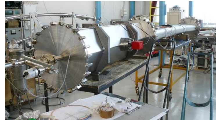
Assembly of dipole and quad chambers prototypes test: nominal vacuum achieved!
