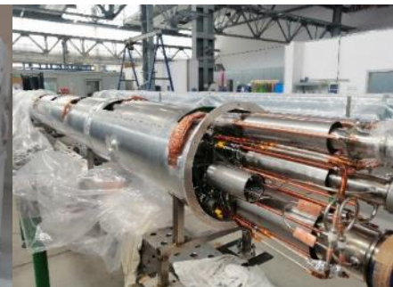
Bypass line at FAT at Kriosystem
