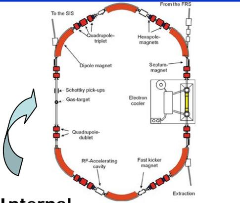
Internal Gas-jet Target
