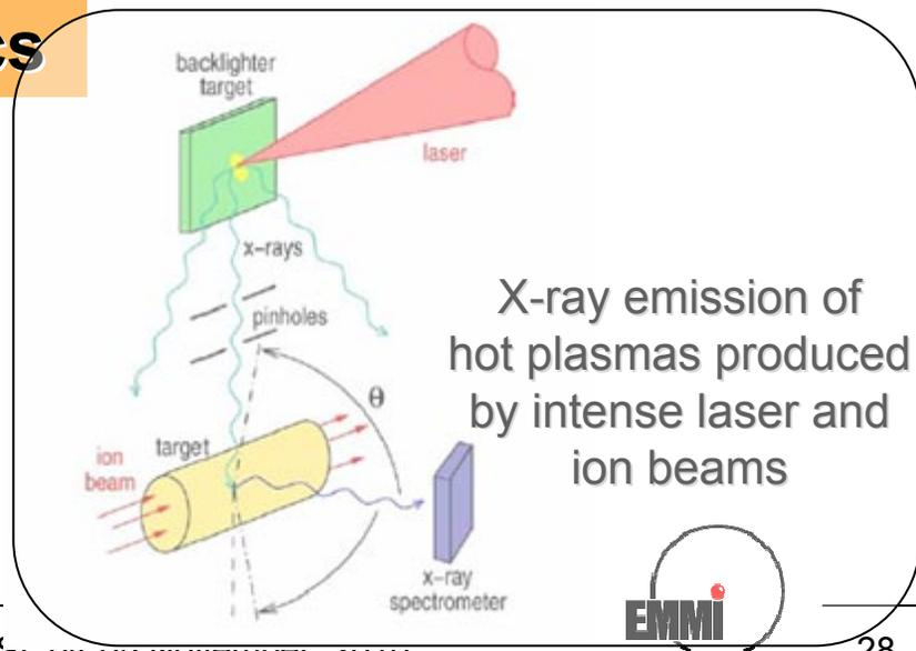
X-ray emission of hot plasmas produced by intense laser and ion beams
