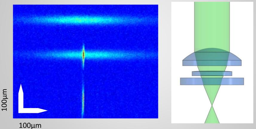
We use the infrared emission of a green laser pointer! (1064nm)
