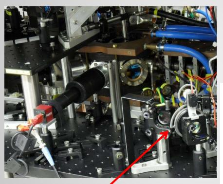
Motorized irises control beam diameter
