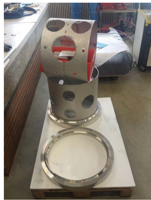
Tank section: In assembly, flange rings t.b. finished after welding
