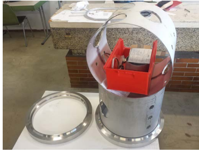
Tank section: In assembly, flange rings t.b. finished after welding
