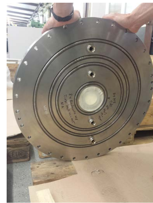
Endplates: Finished, QA -> minor reworking
