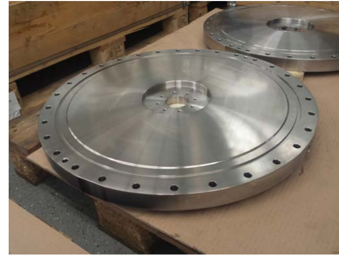
Endplates: Finished, QA -> minor reworking
