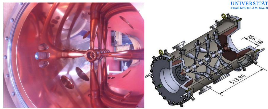
High Field CH - cavity: Built from BMBF funds, fully equipped. Still waiting for the GSI 3 MW Klystron test stand to find out:
