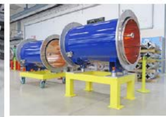
From left to right: dipole magnet, quadrupole lenses, cryostats and vacuum beam pipe of the Collider.
