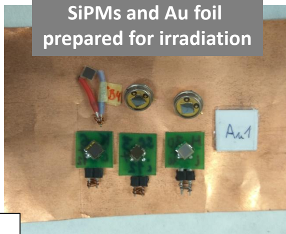
SiPMs located at the holder
