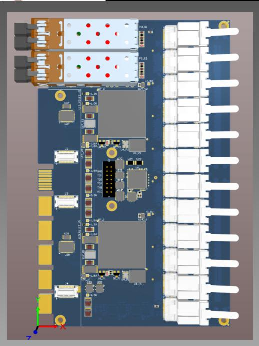
**Readout Board** obtained from the 64-channel ADC for the EMC Forward Endcap
