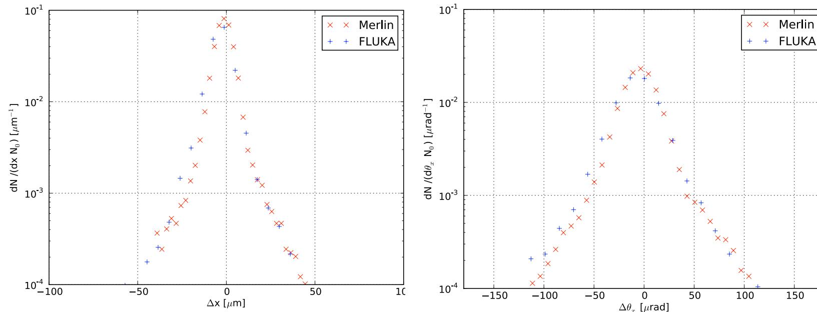
The distribution of change in proton position and direction after scattering through 0.5 m of Copper collimator (IPAC10 Proceedings, TUPD061 )
