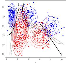
Points from blue and red class are generated by a mixture of Gaussians. Black curve shows optimal separation in a Bayes sense. Gray curve shows neural network separation of two independent backpropagation learning runs.
