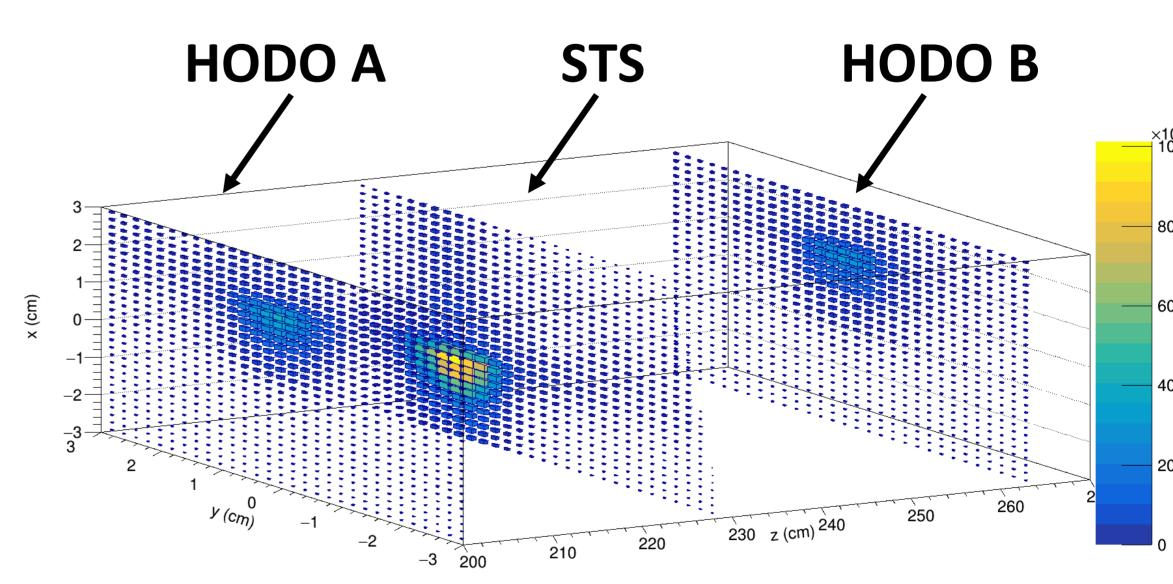
STS sensor displaced in x and y
