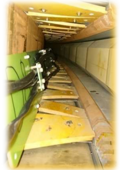
Scintillators installed along vacuum chamber inside dipole
