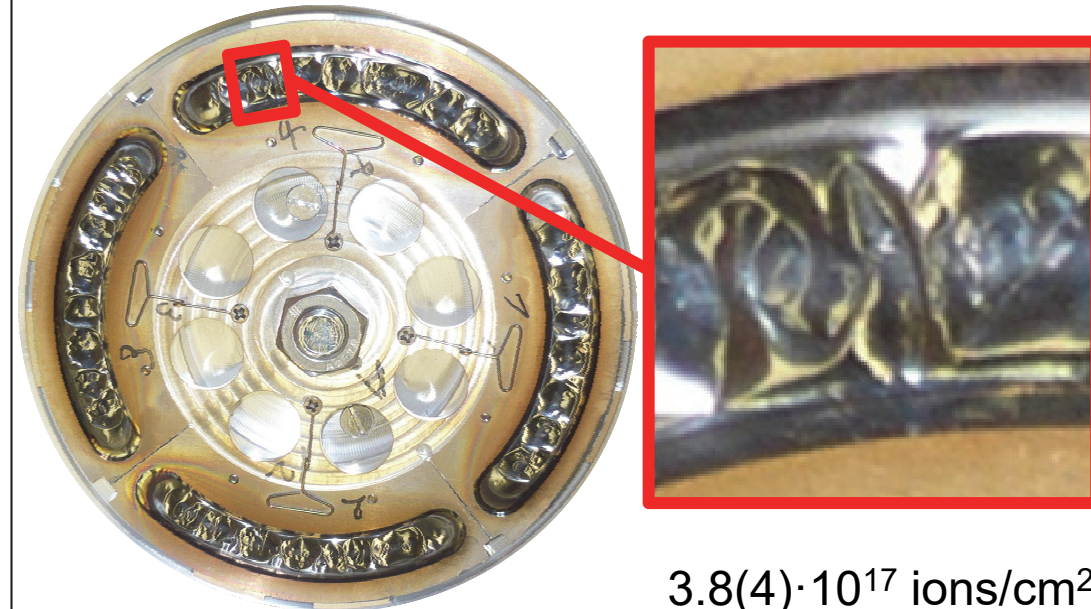
After irradiation ( 9.2 \cdot 10^{18} ^{48}\text{Ca} ions) (intensity: \approx 3-6 \cdot 10^{12} \text{ s}^{-1} // \approx 0.5-1.0 \mu\text{A}_{\text{part}} )
