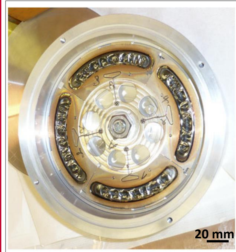
The ^{249}\text{Cf} target wheel after the bombardment with the ^{50}\text{Ti} beam dose of 4 \times 10^{17} ions/cm ^2
