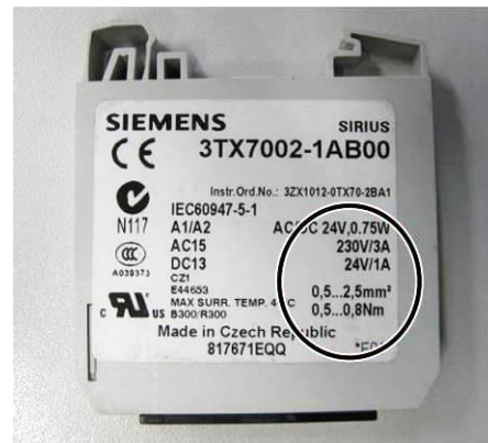
Fig. 84: Torque indications on terminal clamp
