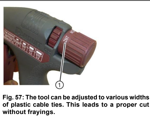
Fig. 56: Cable tie tool for cutting plastic cable ties
