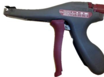
Fig. 36: Cable tie tool for cutting plastic cable ties avoids sharp edges. Cable ties must not be shortened with a wire cutter.
