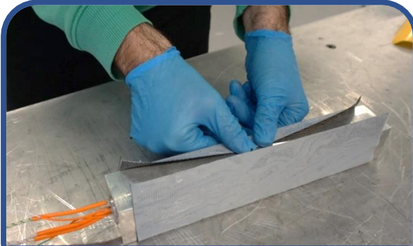
Wrapping mandrel with prepreg
