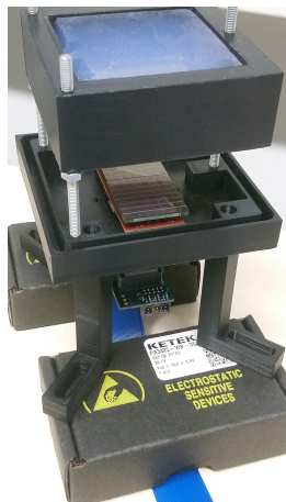
Figure: Test setup with SiPM-Array and aerogel radiator.
