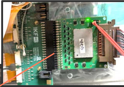
ASIC test board for MDC FEE upgrade
