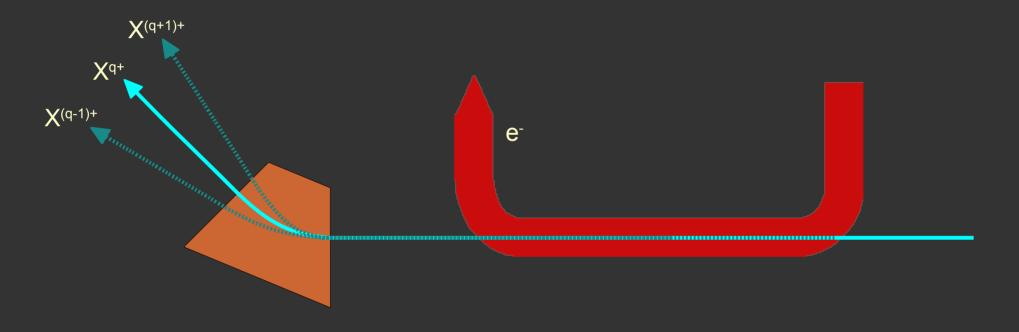
A downstream dipole separates products by charge state. Fast scintillation  $^{DR}$  / CEM detector allow single particle detection with  $\epsilon$ =1
